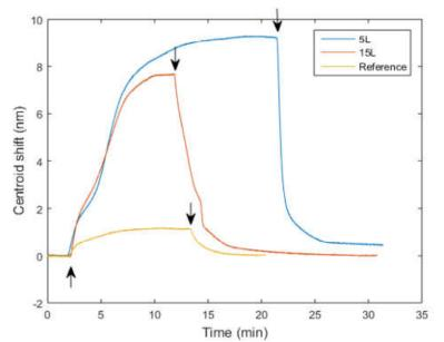
Figur 2. Centroid shift as a function of time and HKUST-1 layer thickness. The first arrow marks the introduction of cyclohexan into the system. The following arrows marks the switch to pure argon.
